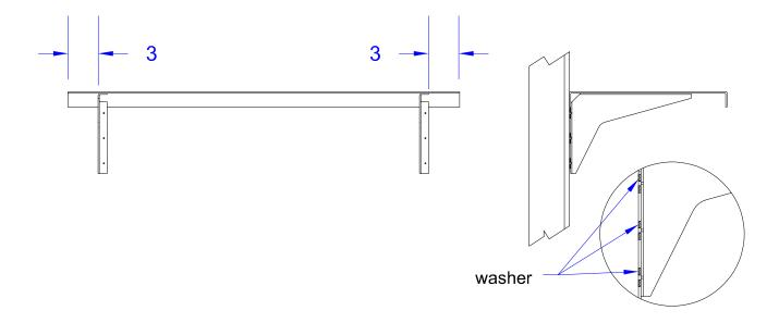
3. When installing on Floor-to-Ceiling posts, put a double sided tape on top of the brackets. and then set the tabletop on that. Secure the table to the 4 FTC posts using self tapping screws so it does not move. You can pre-drill it as well using 1/8" drill bit if you prefer.
